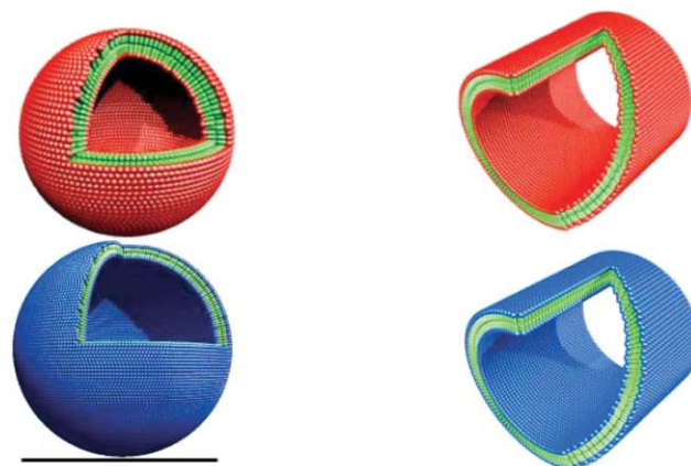
Fig. 5 Molecular models of lipid-like peptide nanostructures. The bilayer structures were determined by neutron scattering with an estimated thickness of 5 nm. 32 Color code: hydrophobic tail, green; red, negatively charged head ( V_6D ); and blue, positively charged head ( V_6K , or KV_6 ). The scale bar is 50 nanometers.
